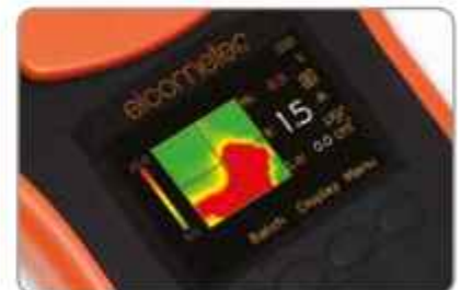
2D Salt Density Map with High/Low Readings
