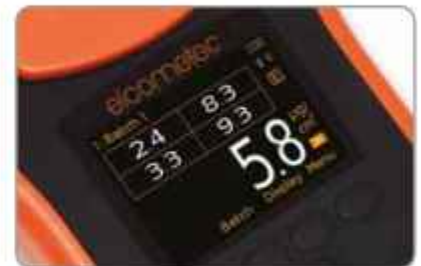
Four Bresle Patch Equivalent Readings
