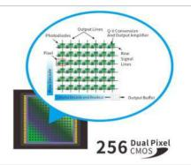
3, 256 Image Element Double Array CMOS Image Sensor
