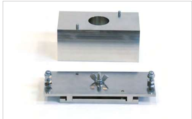
Sand Paper Holder Weight (8118) and Sandpaper Holder (5058)
