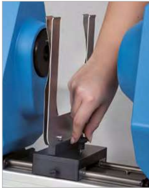
Sample holder for films and sheets. The precision guide carriage allows easy replacement of different holders.
