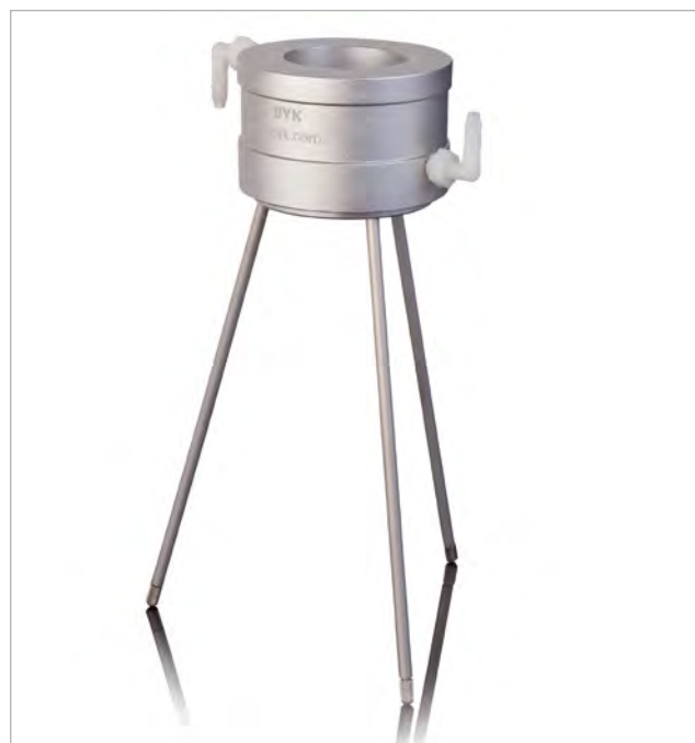
Flow Cup Stand with water jacket - 7210
