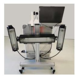
To capture data of light and thermal waves passing into and out of the material, we use a **high-performance IR thermographic camera** capable of capturing temperature modulations from the entire observed body surface at once. On the basis of taken images, the patented algorithm of CarScan software, performs amplitude and phase processing of the temperature path. Using the "Fourier Analysis" algorithm, each pixel is processed individually for each recorded image.
