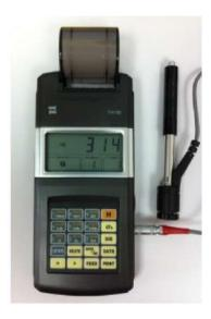
This hardness tester unit has a user-friendly membrane and a built-in mini printer. Hardness scale, material, average time can be set with one touch.
