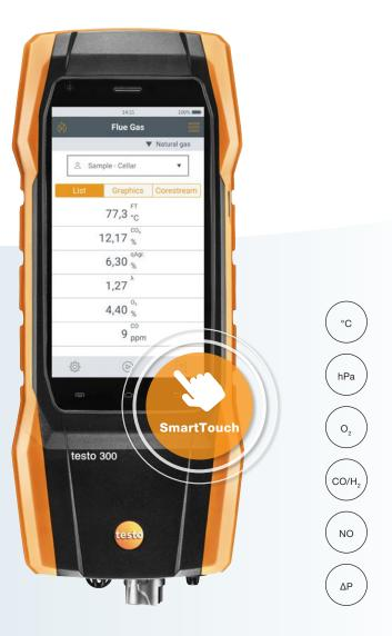
Flue gas measurement truly smart: that is what the testo 300 stands for. The compact flue gas analyzer is fully operated via the large touch display. You can see all the measuring values straight away on this without scrolling. The particularly scratch-resistant screen in embedded in a robust plastic housing which remains reliable even in tough day-to-day working conditions.
