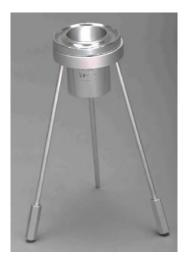
The Flow Cup Stands are precision engineered to ensure the required stability when performing a viscosity flow cup test. We have two options to choose from.
