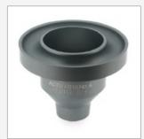
The process of flow through an orifice can often be used as a relative measurement and classification of viscosity. This measured kinematic viscosity is generally expressed in seconds of flow time which can be converted into Centistokes using a viscosity disc calculator. Viscosity Flow Cups are used for measuring the consistency of paints, varnishes and other similar products.
