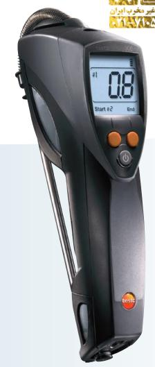
The measuring instrument testo 308 is designed for easy electronic smoke count measurement. It determines the smoke count to one decimal position by constant sampling. The powerful LED backlighting guarantees good legibility even in unfavourable light conditions.
