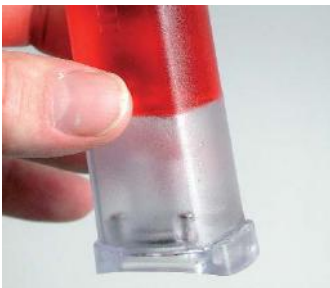
The potassium chloride solution bonded in the gel cannot leak.
