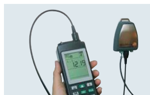
Inspection of transmitters with 4 to 20 mA interface
