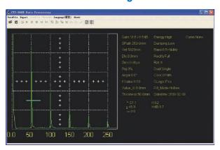
Detection echoes, curves or parameters may be losslessly stored to a PC via the USB port, facilitating report editing and data management.
