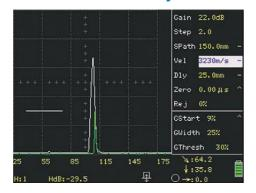
Refresh the highest echo within the screen range automatically, completing flaw positioning quickly.
