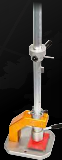
Elcometer 1615 Variable Impact Tester
