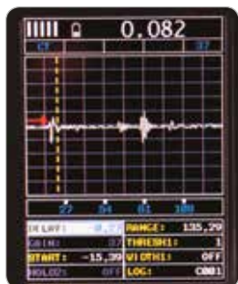
CT Coating Only Mode Displays the thickness of the coating applied to the material.
