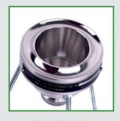
Viscosity cups - testing devices that intended for measurement of rheological characteristics of liquid substances.
