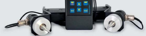
Also it has: mode of the signal visualization (A-scan), the ability of testing concrete (and other) constructions for internal defects and discontinuities, also increases the accuracy of measuring time intervals by manual timing of the moment activation of measurer.
