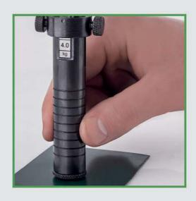
Scratch Hardness Coating Tester NOVOTEST SH-1518 (ball type) is used for hardness testing of coatings (paint, mastic, plastic and others) through determining the hardness resistance to indentation of the ball tip with 1 mm diameter.
