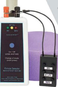
The electrolytic flaw detector (detector of porosity) NOVOTEST ED-3D is designed for rapid non-destructive testing of continuity of coating thickness up to 500 µm in accordance with standard **ASTM G62-A**.
