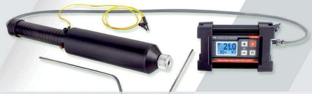
NOVOTEST SPARK-1 is designed according to **ASTM G62-**07, ISO 2746:1998 & AS3894.1-2002, ANSI/AWWAC214-07, ANSI/AWWA C213-07, ASTM D4787-08, NACE RP0274-2004, NACE RP0490-2007, NACE SP0188-2006 for testing the continuity of insulation coatings (polymer, epoxy, bitumen, etc.) of pipelines (oil, gas, etc.) and other products.
