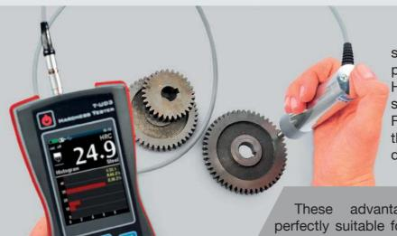
The using of diamond indenter allows setting the probe precisely in any tiny point. The depth of the imprint left by Hardness tester T-U3 is many times smaller than imprint left by standard Rockwell hardness tester, which makes this method of measuring the least destructive.
