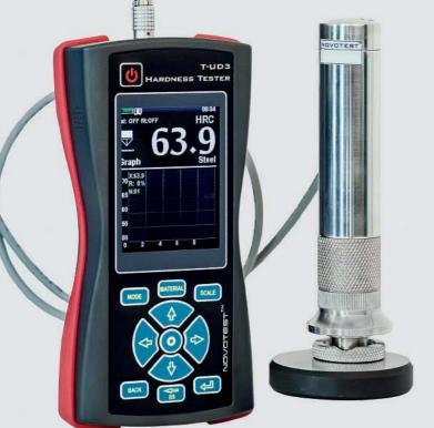
UCI Hardness Tester NOVOTEST T-U3 uses ultrasonic contact-impedance method of measuring hardness standardized according to **ASTM A1038**.
