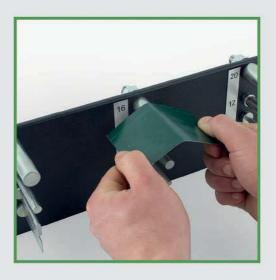
NOVOTEST BEND-H1519 complies with ISO 1519-73, ASTM D 522, ISO6860 which applies to paints and varnishes and describe by method for determining the elasticity of the film bending.
