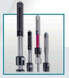
Standard set of Hardness tester includes D type Leeb probe, but it also can be equipped with DC, DL, D+15, C, G, E type probes.
