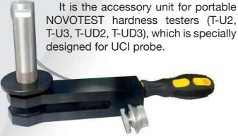
UCI Probe Test Stand NOVOTEST is used for fixation of small, thin products (even less 1 mm) during tests. It makes testing more accurate and more convenient for users.
