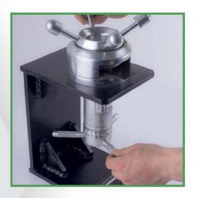
Erichsen Cuppinng Tester is designed for testing of elasticity and strength of coatings with cup-shaped curve, according to **ISO 1520, ISO 20482:2013**.
