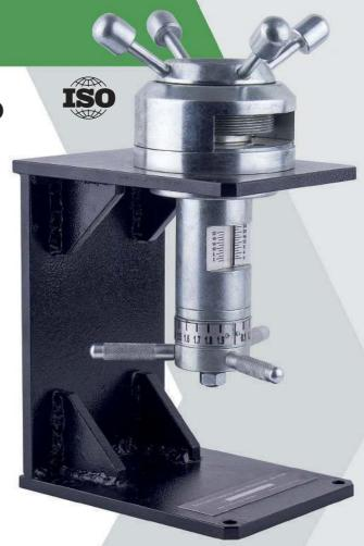
The Ericksen's device is used for determining the strength of the coating at the indentation of spherical tip punch with diameter of 20 mm in the coating of the sample, the position of which is fixed on a matrix with internal diameter of 27 mm.
