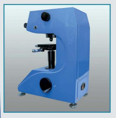
The machine allows user to maximize the efficiency of the using portable hardness testers, especially UCI hardness testers, because TC-MCV-1A implements direct method of hardness measuring.
