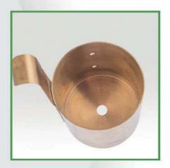
Viscosity Dip Mug is used to determine the convectional viscosity of the dispersion polyvinylacetate homopolymer coarse dispersion.
