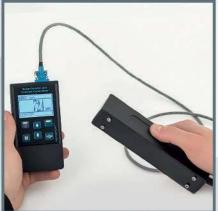
Concrete Cover Meter NOVOTEST Rebar Detector works in a mode of constant scanning of the test surface.
