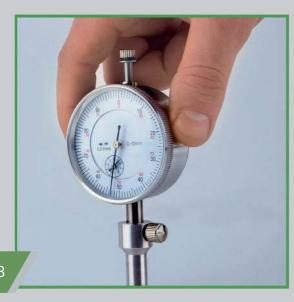
It is used for (depending on configuration): measures the peak-to-valley height of a blast cleaned surface; measurement the depth of focal corrosion; measures depth of narrow holes and grooves.
