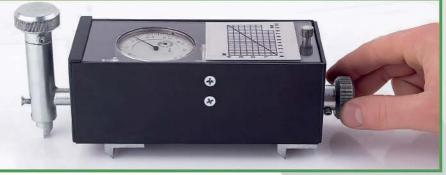
Adhesion tester CM-4219 is a device for measuring the adhesion value of bitumen pipe insulation and other insulating coatings which are based on bitumen.
