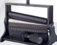
The NOVOTEST BEND-6860 is used to determine the elasticity or resistance, adhesion and elongation of coatings on sheet metal in accordance with **ISO 6860**, **ASTM D 522-A, BS 3900-E11, ECCA T7.**
