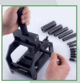
The device complies with **ISO 1519-73**, **DIN 53 152** and applies to paints and specifies a method for determining the elasticity of the film by bending. The device allows to measure the elasticity and strength of coatings through bending the metal plate with tested coating around a set of cylindrical rods with diameters from 2 mm to 32 mm.
