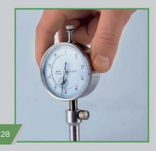
It is used for (depending on configuration): measures the peak-to-valley height of a blast cleaned surface; measurement the depth of focal corrosion; measures depth of narrow holes and grooves.
