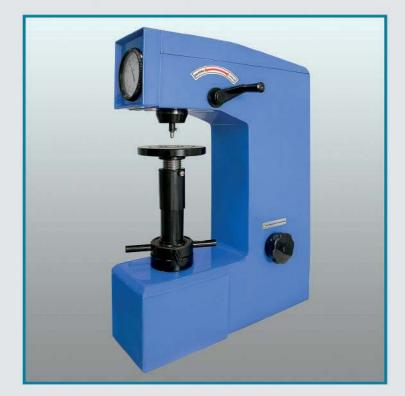
NOVOTEST TB-R implements direct Rockwell method of hardness testing, which is based on the testing of samples for resistance to penetration of indenter with certain load – the most commonly used hardness test method.
