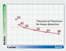
Contrast (signal) of all films is optimized to approach the maximum contrast for a linear detector (industrial X-ray Film), thereby optimizing image quality and perceptibility. An exception to the rule is D2, a super linear detector, where image quality is optimized through more than linear (extremely high) contrast in combination with very low noise.
