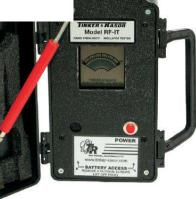
The RF-IT emits an audible beep. When the operator gets closer to the point of contact the unit starts beeping faster. At the same time, the LCD meter moves from left to right.
