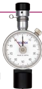
GS-719P GS-709P Type A Durometer Peak pointer type
