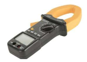
DT-3310 Series Professional 1000A AC Clamp Meters provide many functions for professional AC current and voltage measurements including resistance, capacitance and diode test, etc. With mid-size and tear-drop shaped jaw, it is easy to use in crowded cable areas and other tight places.
