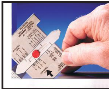
CHECK THE THROAT OF FILLET WELD
